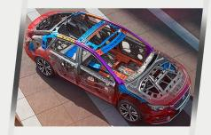
The MG 6 is built around an ultra-rigid safety cage and features a 6-airbag system.
